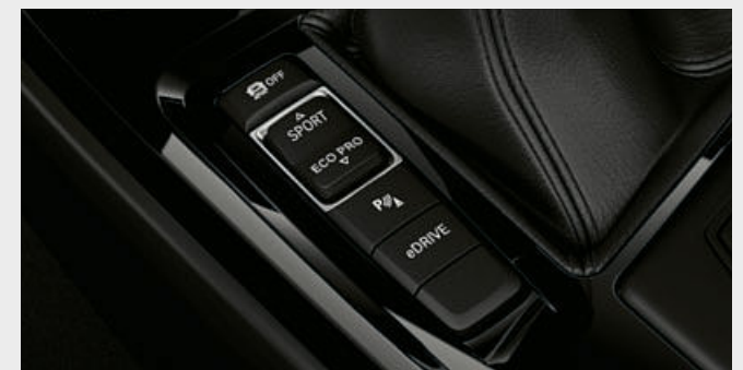
With the driving mode button in the centre console, the AUTO eDrive, MAX eDrive and SAVE BATTERY driving modes can be selected intuitively. At the touch of a button, the driver can quickly adjust the plug-in hybrid drive to different driving situations.
