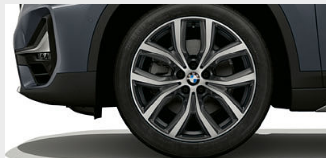
□ 19" light alloy wheels Y-spoke style 511 Orbit Grey, gloss-lathed, wheel size 8J x 19 with 225/45 R19 tyres.
